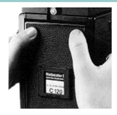
**4.** Close the back cover. When closing the back cover, firmly press both sides at the upper portions of the back cover as indicated in the photo.
